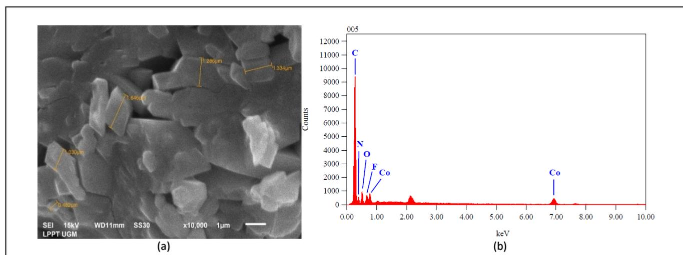
**Figure 4.** SEM photograph of  $[\text{Co}(\text{bipy})_3](\text{CF}_3\text{COO})_2 \cdot 5.5\text{H}_2\text{O}$  at a magnification of  $10,000 \times$  showing crystal size (a) and EDX showing elemental content (b)
