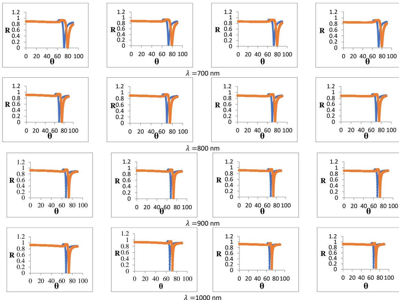
**Figure 3.** Reflectance of the suggested sample with incidence light angle for different wavelengths ( $\lambda=100-1000$  nm) and different  $Ta_2O_5$  layer thicknesses (a)  $d=0$  nm, (b)  $d=25$  nm, (c)  $d=50$  nm, and (d)  $d=75$  nm. The blue line is  $\Delta n_m = 0$ , and red line  $\Delta n_m = 0.04$
