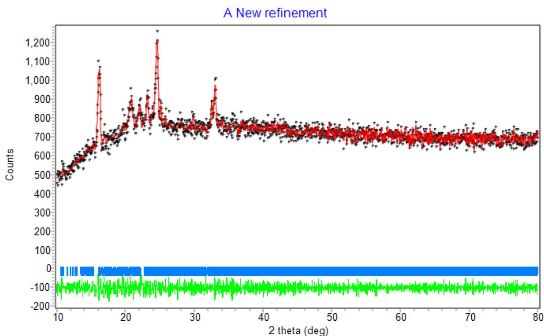
**Figure 5.** P-XRD profile of  $[\text{Co}(\text{bipy})_3](\text{CF}_3\text{COO})_2 \cdot 5.5\text{H}_2\text{O}$  (black), the monoclinic symmetry of C2/c due to the refinement (red), the position of  $2\theta$  (blue), and the difference between the two (green)
