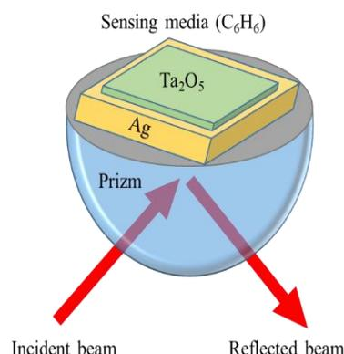
**Figure 1.** The schematic diagram of the SPR system based on the Kretschmann configuration.
