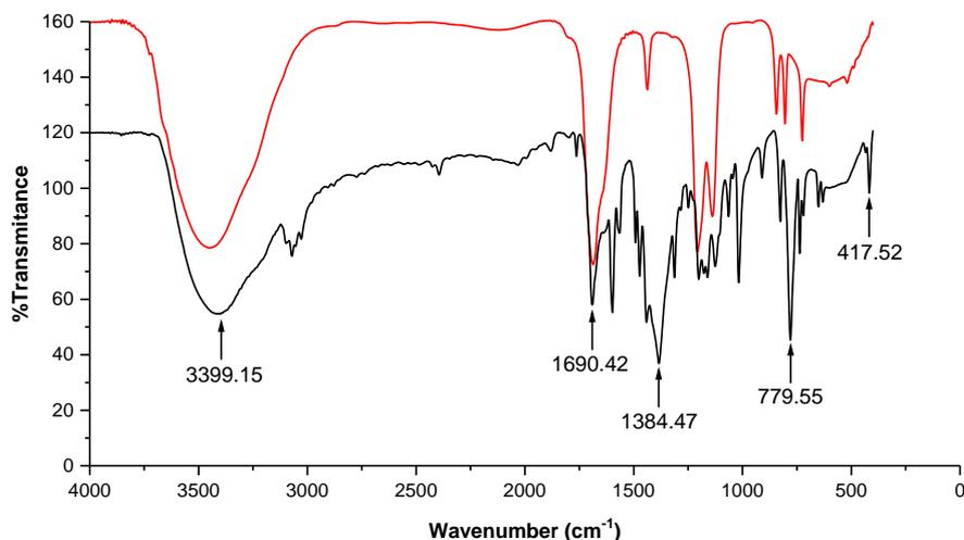
Figure 3. The IR Spectra of  $[Co(bipy)_3](CF_3COO)_2 \cdot 5.5H_2O$  (black) and  $CF_3COONa$  (red) [Note: Relative transmittance (in %) only significant for each spectrum]
