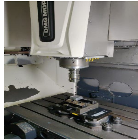
Fig. 6. Experimental set-up of the milling of a sample specimen
